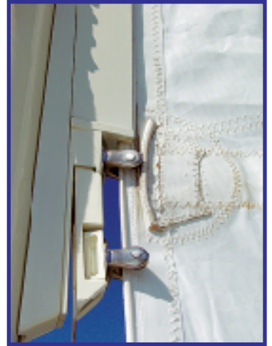
Sail track with one-piece PVC runner and self-guiding feeder
