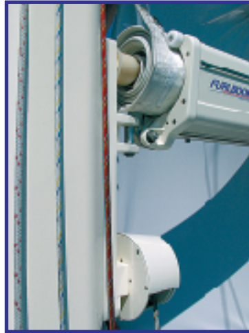
Open front prevents sail jamming
