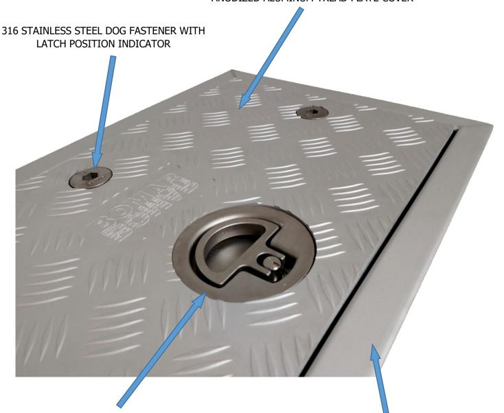
316 STAINLESS STEEL FLUSH D HANDLE FOR EASY REMOVAL AND REPLACEMENT OF HATCH COVER HEAVY 12 GAGE 316 STAINLESS STEEL FULLY WELDED FRAME CAN BE DIRECT BONDED OR MECHANICALLY FASTENED (ALUMINUM FRAME IS OPTIONAL FOR DIRECT WELDING TO ALUMINUM DECK)
